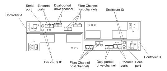
Figure 3. Back view; controllers with two standard and two optional Fibre Channel host expansion channels
